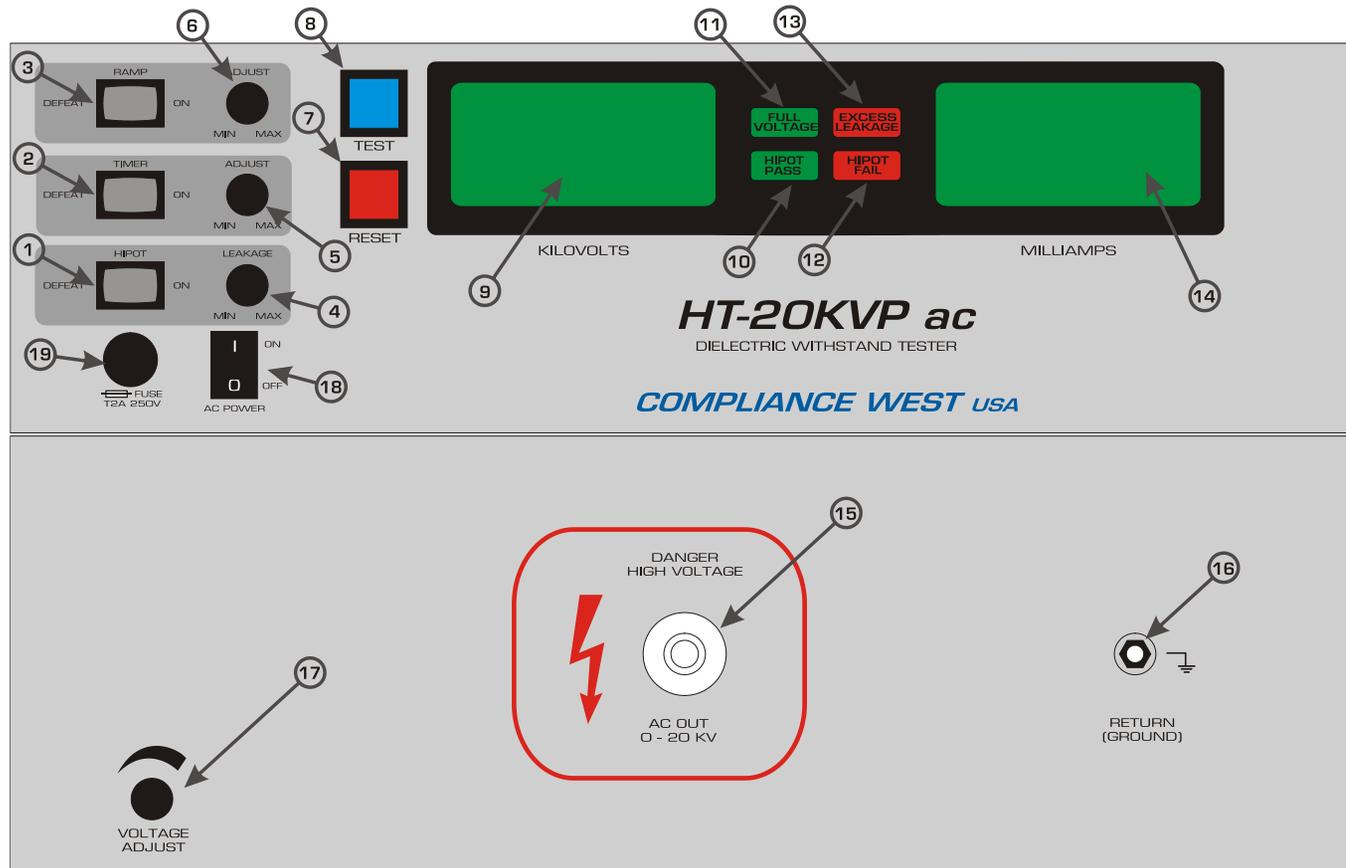
**Figure 4-1. Front Panel Controls, Indicators and Connectors**
